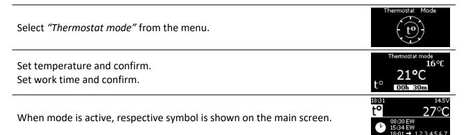
Default value for MAX temperature rise is 1°C and MIN temperature drop is 2°C. These settings can be changed in "Settings -> Heater -> Advanced -> Thermostat".
